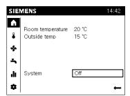
Use **plant/zone switch** "Off" if you leave your house or apartment for an extended period of time. The building is protected. Energy consumption is reduced to a minimum. Set upon return to "Automatic", and the entire plant returns to operation.
