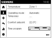
Use the **time program** to operate the building or living zones at a reduced temperature during daily vacancies or at night. The time program is used only in operating mode Automatic.
