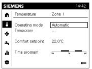
As a rule, the **operating mode** is set to Automatic: In this mode, the controller works correctly and uses all available energy saving options (e.g. summer/winter mode).
